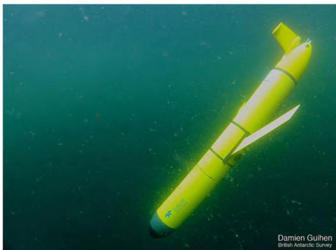
*A Teledyne Webb shallow-water slocum glider in action, operated by NOC. This vehicle is fitted with a 120kHz echosounder and can be used to image fish shoals and zooplankton aggregations. Photo: Damien Guihen (British Antarctic Survey, UK).*
