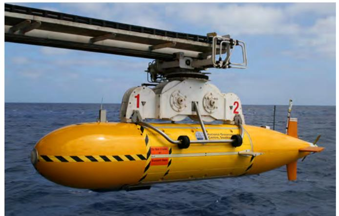
*The Natural Environment Research Council (NERC) Autosub6000 AUV, which operates down to 6000 m and is used for a wide variety of seafloor mapping and oceanographic applications. Photo: R. Wynn.*
